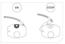
If your cylinder is pierced or your lever is not in the up-and-ready position with the green indicator pin in place, you will need to re-arm your flotation device (see Re-arming, p. 11) before continuing.
